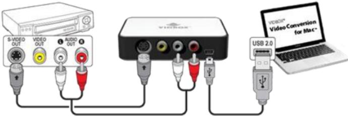
**Tip:** It is important to connect the capture device to your computer before opening the Video Conversion for Mac application, to ensure proper device detection.
