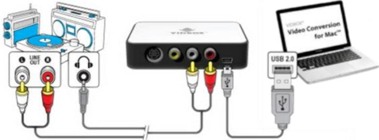
Connections from your audio player can be made via **RCA stereo cables** or with a **Headphone-to-RCA stereo adapter cable (not included)**.
