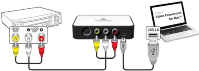
Connections from your video player can be made via **RCA composite video and audio cables** (above), or with a combination of **S-Video and RCA stereo audio cables** (below).
